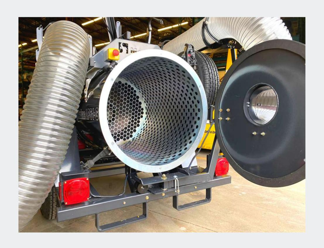
Increase LP61-G litter container capacity from 0.3 cu. yd. to 4 cu. yd. (1233% increase) with the Madvac LC400, or 6 cu. yd. (1900% increase) with the Madvac LC600.
